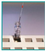
Insert capillary in an HB 142 cuvette
