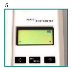
Switch on photometer Press Enter Select test "HB" with arrow key Confirm with Enter
