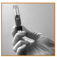
**2.** Screw on cap Turn cuvette upside down several times
