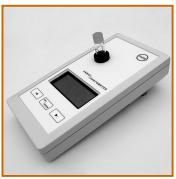
**8.** Read the measured value of cuvette 1, remove cuvette Insert cuvette 2, read the measuring value, remove cuvette etc.
