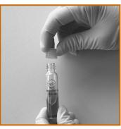
**5.** After blank adjustment of the last cuvette replace all screw caps against starter caps
