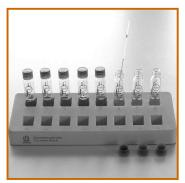
**1.** Wash out samples from capillaries into cuvettes with micropipetter
