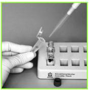
3. Insert 500 µL sample in each cuvette Note: Work on each cuvette individually and return it immediately in the thermostat to avoid cooling.
