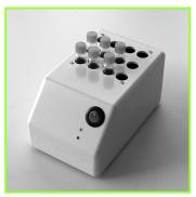
**4.** After pipetting the last sample, incubate cuvettes exactly for 1 minute Meanwhile switch on photometer
