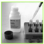
1. Pipette 1 mL buffer solution in each cuvette Close cuvettes
