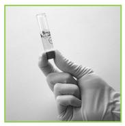
4. Screw on cap and turn cuvette upside down several times
