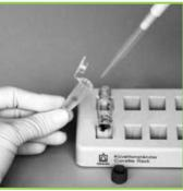
3. Remove 500 µL supernatant from the reaction tube "R" and transfer it into a cuvette
