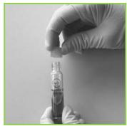
7. Replace screw cap against starter cap Turn cuvette upside down
