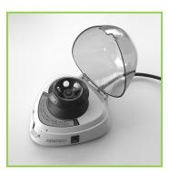
2. Insert reaction tube "R" with capillary into centrifuge Centrifugate 1 minute Hint: Pay attention to an even load of the centrifuge!
