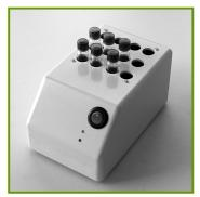
**1.** Incubate cuvettes in preheated thermostat for 7 minutes
