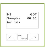
**5.** Start measurement with ON/ENTER Time (1 minute) counts down, cuvettes remain in thermostat
