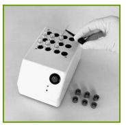
2. Insert 50 µL of sample with e-t-e capillary in each cuvette Do not mix yet!
