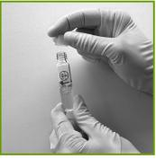
**3.** Screw on starter cap and mix well Insert in thermostat immediately
