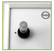
**6.** Note: When inserting the cuvette, the capillary must be placed on the side of the cuvette and right on the black arrow, so that the measurement is not disturbed by the capillary
