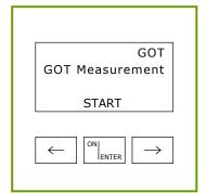
**4.** Switch on photometer with ON/ ENTER
