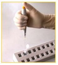
Add 20µL sample (biodiesel) at polystyrene pearls and wash out the capillary with reagent solution with micropipettor
