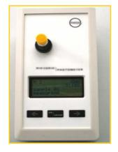
Afterwards insert cuvette in photometer
