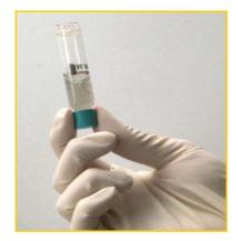
Screw on turquoisecoloured cap again Mix the cuvette thoroughly Wait for 1 min.
