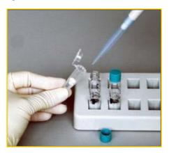
Pipette 500µL aqueous solution in a GLY 742 cuvette
