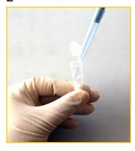
Pipette 1000µL dest. water in reaction tube
