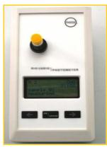
Afterwards insert cuvette in photometer Wait for result
