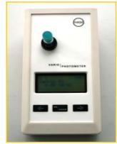
Insert cuvette with biodiesel sample in photometer (blank value); photometer saves blank value
