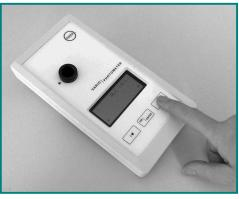
**2. Select test:**Press arrow key until required test appears
