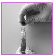
**2.** Screw on control cap on the cuvette that is to be tested
