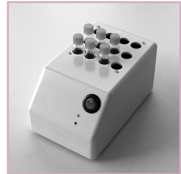
3. Close cuvettes, mix and insert into thermostat immediately
