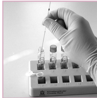
2. Insert 20 µL serum/plasma into cuvette
