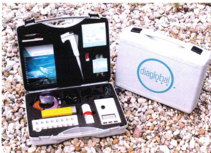
Fig.1. Mobile photometric laboratory of the German company Diaglobal GmbH.
